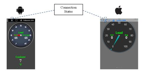
The Connection status screen shows the status of the Bluetooth connection, and allows the selection of a given UltraGauge Blue<sup>™</sup> Adapter, if multiple Adapters are paired.
