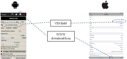
UltraGauge can attempt to retrieve this information automatically or it can be entered manually. To use automatic configuration, there must be a valid VIN displayed in the "VIN" field. If UltraGauge was able to retrieve this information from your vehicle, a valid VIN (similar to the one shown above) will be displayed in this field. If not, "Unknown" is displayed. If "Unknown" is displayed, manually enter the vehicle's VIN.
