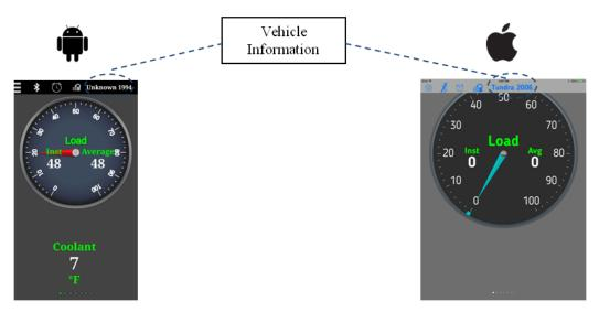
The Vehicle Information screen displays the model name of the vehicle along with other detailed information. To optimize the information gathered by UltraGauge, the following fields should be completed automatically or manually:
