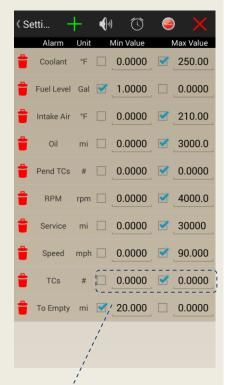
To edit an existing alarm, modify the Min/Max value or check box from the Alarm Enable screen. To delete an existing alarm, select the trashcan next to the alarm you would like to remove.
