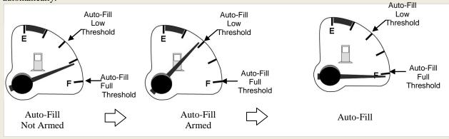
By default the Low Threshold is set to 50% and the full threshold is set to 98%. Setting the Low Threshold too high may cause a false Auto-Fill event to trigger as a result of gas sloshing around in the fuel tank.
